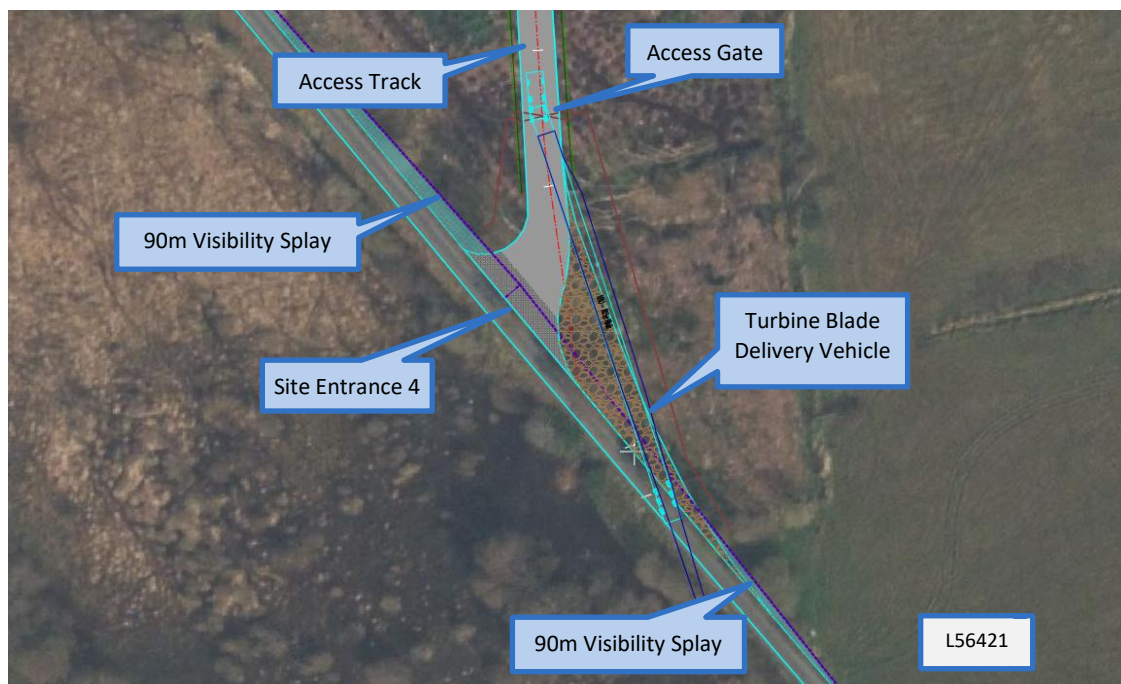
Figure 9 – Site Entrance 4 on the L56421
