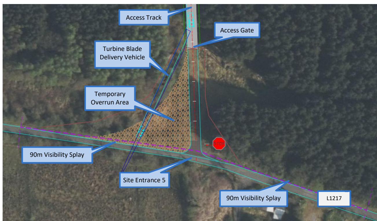
Figure 10 – Site Entrance 5 on the L1217
